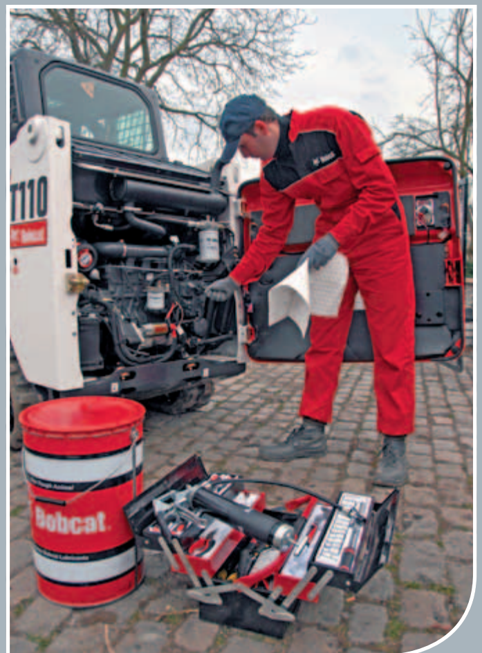
Transverse-mounted engine and swing open tailgate offer increased ease of maintenance.
